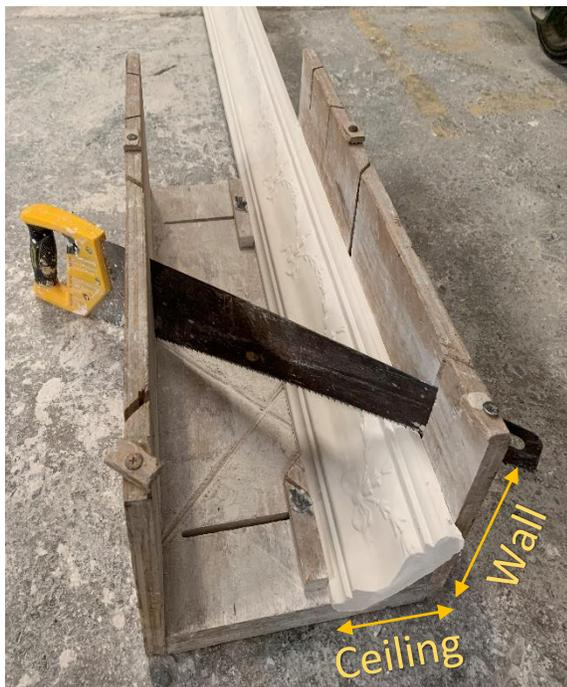
Set cornice ceiling projection on base of the mitre box with guide nails as shown to hold cornice in the correct position while cutting mitres. **This is important for the mitres to fit accurately!**
